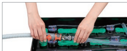
Refilling preparation: Snap-connect the couplings of the hoses on the tank and battery sides and open the faucet.
